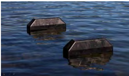
Floats stay at the waterline as you drop your trailer into the water
