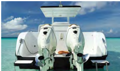
Dual cut out patterns for boats with side by side mount dual outboards - cut out opening in stern section is 50"
