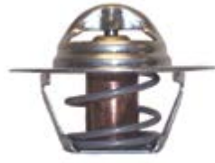
18-3551 THERMOSTAT Replaces: R026002E 142° For: FORD 302/351 CID Engines Raw Water Cooled
