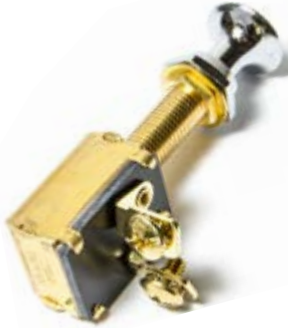
MP39530** MP39532 (Bulk 100pcs/carton) OFF-ON SPST • Pull for ON • Solid brass construction • 3/8" mounting bushing • 2 screw terminals • For panels up to 1" thick • Chrome plated solid brass knob • Rated: 15 amp @ 12 VDC
