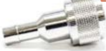
18-80401 FUEL CONNECTOR Female hose connector, new style, 3/8" hose, Will not interchange with OE's 5/16" hose assemblies. Mates with 18-80400 , tank outlet
