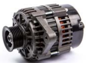
18-5984 ALTERNATOR Replaces: 575011 75I/70 amp, Spool Mount, Serpentine Pulley
