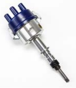
18-26110-1 DISTRIBUTOR Replaces: 9-26110; Mallory YL579AV For: Chrysler V8, 273, 318 (1967 & Up), 340 and 360 "LA" Engines
