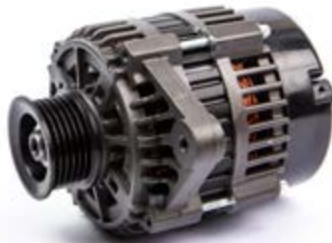
18-5984 ALTERNATOR Replaces: RA097007B 7SI/70 amp, spool mount, 2 5/8" OD, 6 groove serpentine pulley Clockwise position, 65mm
