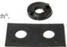
MP78960 MP78962 (BULK 100 PCS/CTN) Anti-rotation collar. Use when installing non-illuminated RotoSwitches in very thin dash panels. This adapter prevents the switch from "slipping" if excessive force is used to actuate the switch.
