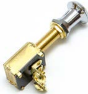
MP39520** MP39522 (Bulk 100pcs/carton) OFF-ON SPST • Pull for ON • Solid brass construction • 3/8" mounting bushing • 2 screw terminals • For panels up to 1" thick • Chrome plated plastic knob • Rated: 15 amp @ 12 VDC
