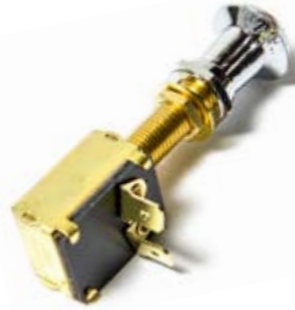
MP39610** MP39612 (Bulk 100pcs/carton) OFF-ON(1)-ON(2&3) SPDT • First pull energizes #1 • Second pull energizes two separate circuits • For anchor/running lights or similar function • Solid brass construction • 3/8" mounting bushing • 4 screw terminals • For panels up to 1" thick • Chrome finish plastic knob • Rated: 15 amp @ 12 VDC
