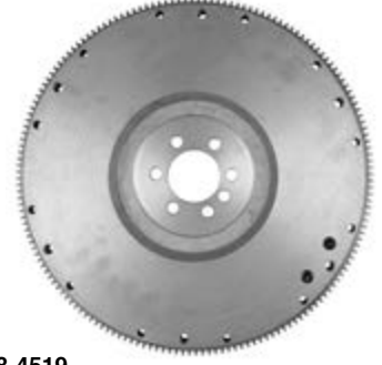
18-4519 FLYWHEEL 14" 5.0/5.7L, 1 piece main 1987 and UP. Bottom mount starter (Block mounted) applications.
