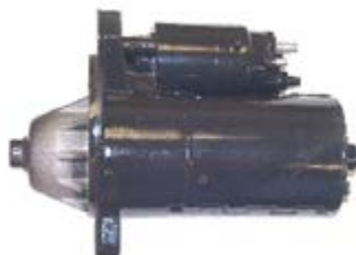
18-5920 STARTER Replaces: 3854190 Clockwise/Standard rotation Permanent magnet starter Replacement Solenoid: 18-6291 For: 5.0 & 5.8 litre Ford engines
