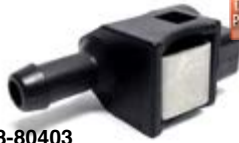
18-80403 FUEL CONNECTOR Female 3/8 hose connector with rectangular locking post, Will not interchange with OE's 5/16" hose assemblies. For late model engine: For use with our 18-81042 fuel hose assembly, motor end. Mates with 18-80407
